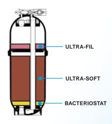
Well Water configuration for hardness and acid neutralization.
